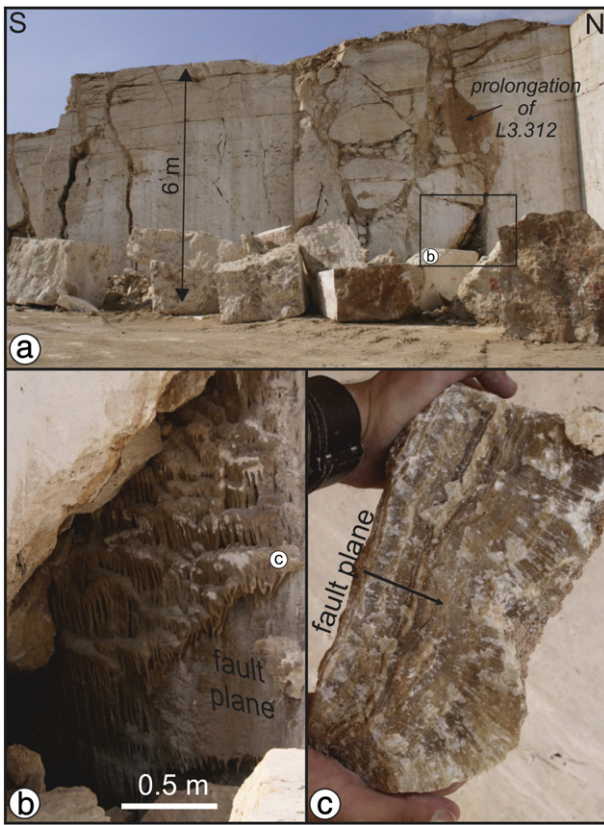
Fig. 7. (a) Irregular high-angle faults in the Abandoned quarry with (b) speleothems at the northern fault wall. The stalactite morphology of the columnar calcite precipitation demonstrates that the precipitation originates from descending fluids. (c) Detail of (b) showing typical colour-banding that locally can reach a thickness of 20 cm.
