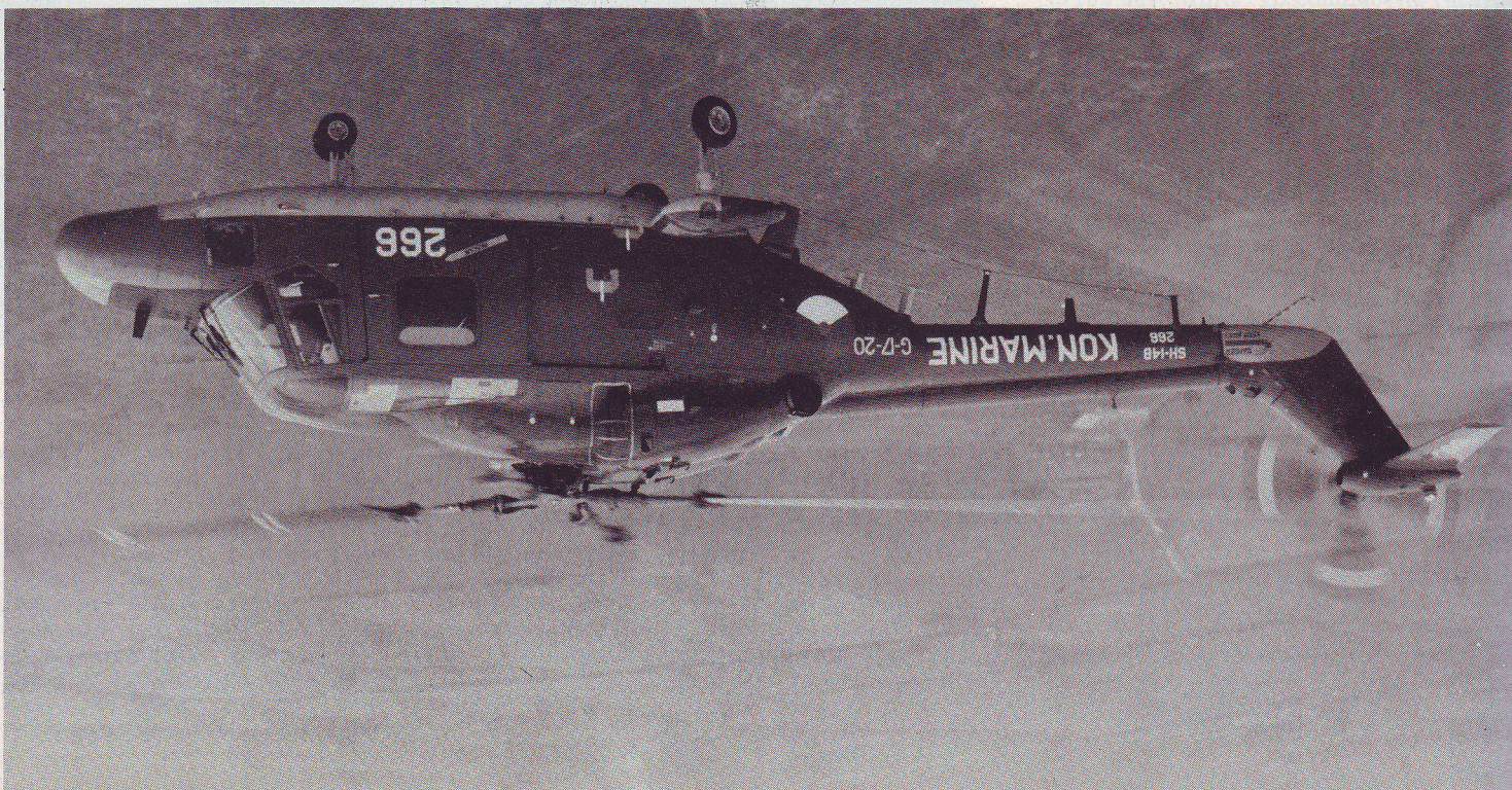
A Westland Lynx helicopter of the Koninklijke Marine. The Dutch Navy has an antisub squadron of 17 SH-14B/C and an SAR squadron with 6 UH-14A, besides other machines to be carried on the naval units.
