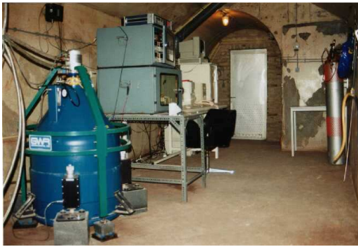
Figure 4 : The superconducting gravimeter GWR#C021 measures continuously the variations of the gravity in Membach with a precision of 10^{-10} g. There are about twenty superconducting gravimeters throughout the world.
