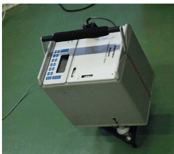
Figure 2 : The spring gravimeter Scintrex CG3M is one of the instruments the Observatory uses in the field. This instrument measures the variations of the gravity with a precision of 10^{-8} g.
