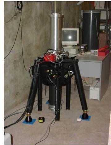
Figure 3 : The absolute gravimeter FG5#202 determines the gravity in Membach with an accuracy of  $10^{-9}$  g. As a function of the seasons, the value of  $g$  varies from 9,810 467 20 to 9,810 470 30 m/s<sup>2</sup>, after correction of the known variable effects such as the tides. Presently there are only some thirty of these instruments in the world.
