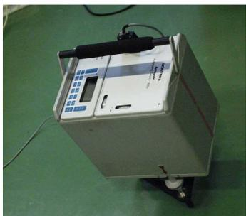
Figure 2 : The spring gravimeter Scintrex CG3M is one of the instruments the Observatory uses in the field. This instrument measures the variations of the gravity with a precision of  $10^{-8}$  g.
