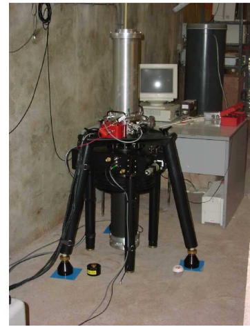
Figure 3 : The absolute gravimeter FG5#202 determines the gravity in Membach with an accuracy of 10^{-9} g. As a function of the seasons, the value of g varies from 9,810 467 20 to 9,810 470 30 m/s 2 , after correction of the known variable effects such as the tides. Presently there are only some thirty of these instruments in the world.
